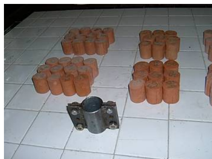
Figure 1 Test brick-cylinders and mould
