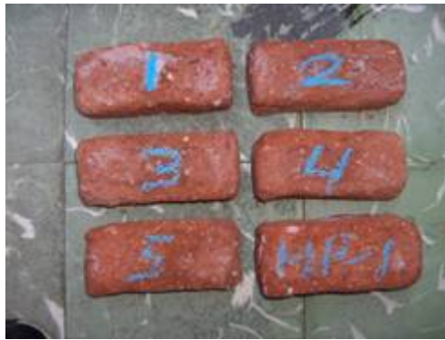
Figure10 Results of salt crystallization tests performed on real bricks
